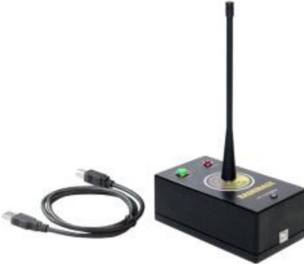
L.S.D. Radiobase is needed to connect the game server (personal computer, laptop) with L.S.D. Electronics game kits. Works by RF. Has the function of starting and stopping the game for all the game kits in the radio visibility zone. This is a green and red button, which respectively activate and deactivate game kits.
